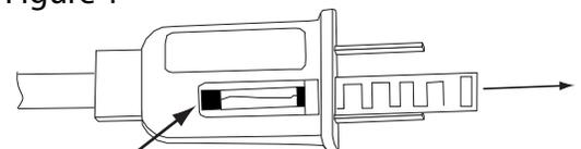
Fuse is inside plug. Slide open or unscrew fuse access cover as shown.
