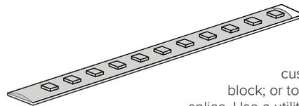
Remove 3/16" of the IP65 protective covering at the end of tape to make custom jumpers using the IP54 4-in-1 connector block; or to use the connector block as a power feed or splice. Use a utility knife to gently cut through the clear jacket, then peel it off carefully using the blade or by hand.
